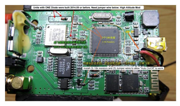
(3) 10k resistors and (3) jumper wires must be added to the radio to allow Auto ON/OFF to work.
