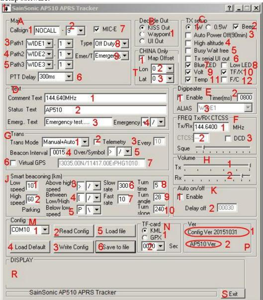
Configuration Description by Section: (Main, Decode Out, CHINA Only, TX setup, Text, Digipeater, Trans, Freq Tx/RX CTCSS, Volume, Smart beaconing (km), Auto on/off, Config, TF-Card, Ver.) (Defaults show in {text box} [check box] |drop down| < radio button>)
