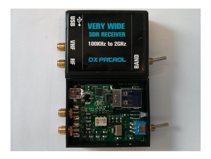
Toggle switch will select the SMA antenna input. The LED light color will indicate.
