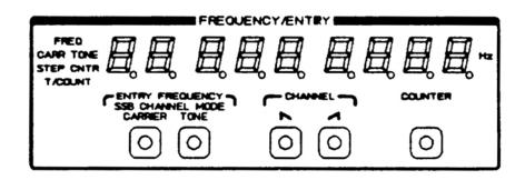
**4.3 Frequency/Entry Group** -On the upper RH side of the front panel is the frequency/entry subpanel. This panel will usually display the frequency that the instrument is tuned to. It will display during frequency entry frequencies being entered by the instrument's keyboard in KHz or Hz. This frequency will be the center RF frequency of the selected band pass filter except when in the SSB channel measurement modes.
