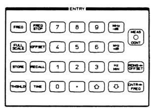
key's red light will turn on or flash indicating the instrument's measurement process has been interrupted. Anytime you see this button's light and want to return to the measurement mode press this key to continue measuring. You can also press it to cancel a mistaken partially keyboard entry.
