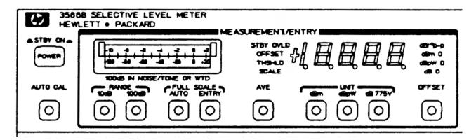
**4.2 Measurement/Entry Group** - On the upper LH is the measurement/entry sub panel, which is used for displaying the power or voltage measurements and their units on a LED display. The measuring range and range full scale range value is set using its buttons. Set the range by pressing [10db] and the full scale range limit by pressing [AUTO] for the automatic mode.
