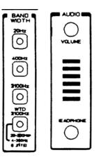
**4.10 Audio Group** -On the lower far right is the audio sub panel. This panel contains a small speaker and headphone jack along with a volume control knob for output of audio from the SSB detector. Since we won't be using the audio output during our first measurements turn the volume knob full CCW to turn off the sound.
