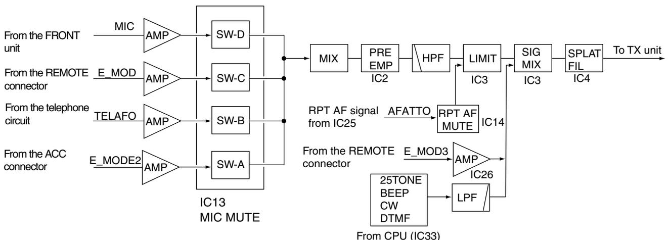
The mixed signals are applied to the splatter filter (IC4).
