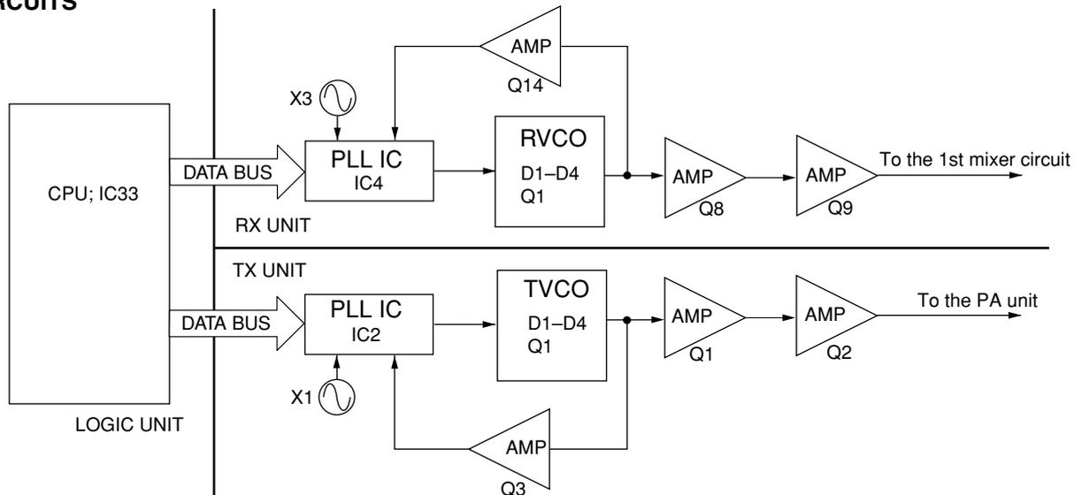
amplifier (Q14) as RX PLL lock voltage.
