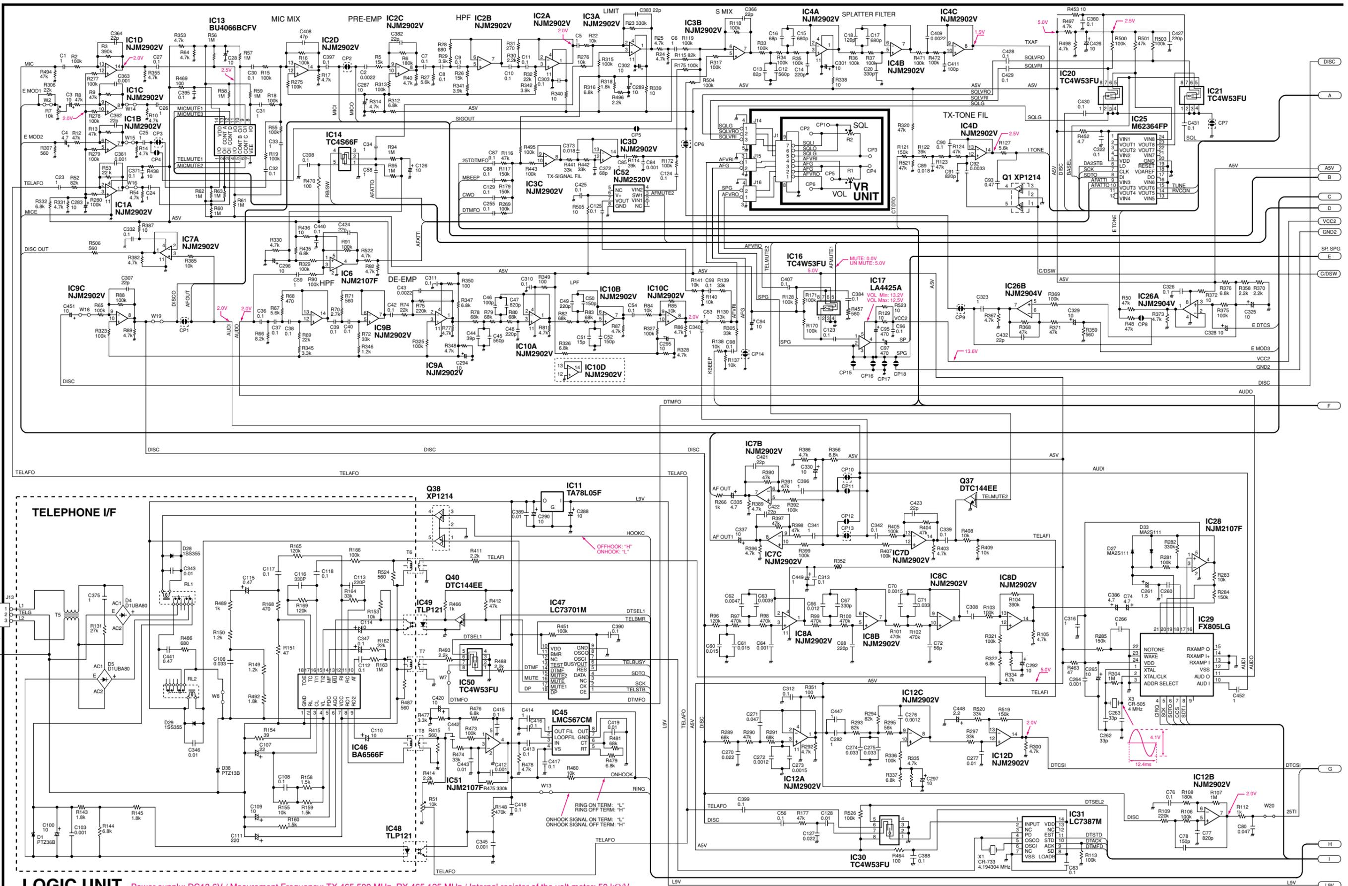
**LOGIC UNIT** Power supply: DC13.6V / Measurement Frequency: TX 465.500 MHz, RX 465.125 MHz / Internal resistor of the volt meter: 50 kΩ/V
