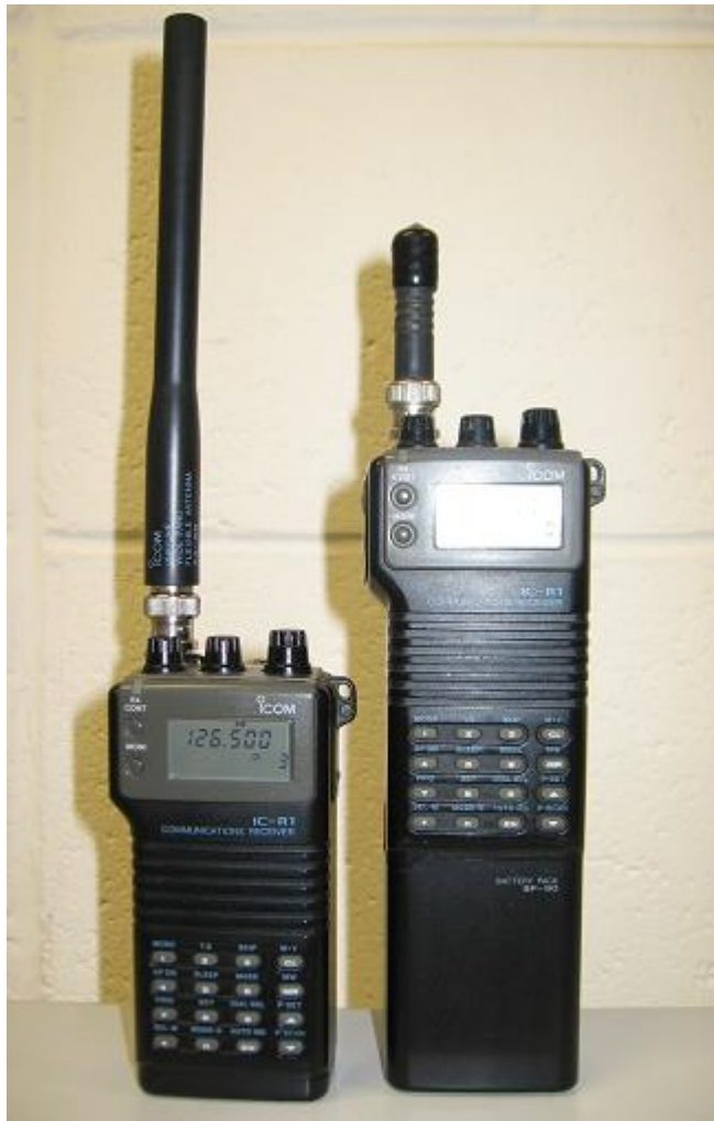
Two Icom IC-R1s: on left with standard FA-4B antenna and no extension battery, on right with optional BC-90 battery case with 6xAA batteries.
