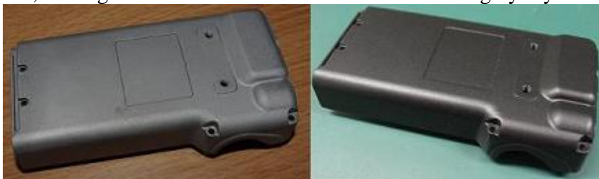
Sand-blasted to bare metal chassis on left, repainted & ready for reassembly on right:
