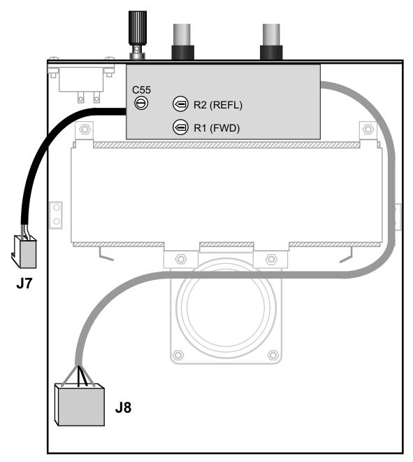
If you have the 160-meter module installed (K160RX), remove its retaining screw and unplug the module. Do not remove the RX Antenna connector or detach the 160-meter module from the heat sink.
