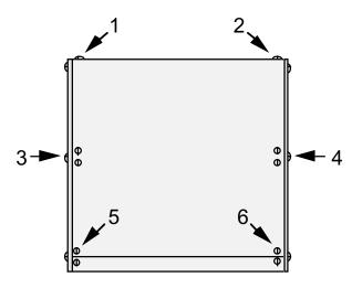
Remove the top cover by lifting it from the back end. Disconnect the speaker and battery cables.
