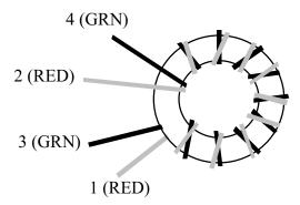
Trim the leads of T1 to about 1/2" (12 mm) long. Completely remove the insulation from T1's leads up to the edge of the core, using a solder pot or hot soldering iron tip. Do not attempt to burn off the insulation using a match or lighter, as the flame may fuse the pairs of wire together, causing them to become shorted. Another way to remove the insulation is to use fine sand paper.
