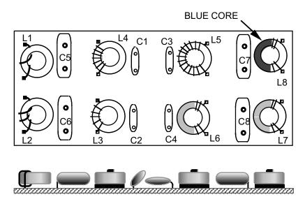
Install C4 (82 pF) as shown above. Trim the leads to about 1/8" (3 mm) long, and bend them down at right angles to the capacitor body. (Adjust the lead spacing to match the pads.) Insert the leads into the C4 pads just far enough to hold the capacitor in place. Do not insert the leads all the way through the board. They could puncture the relay on the opposite side **during soldering, causing a short.**
