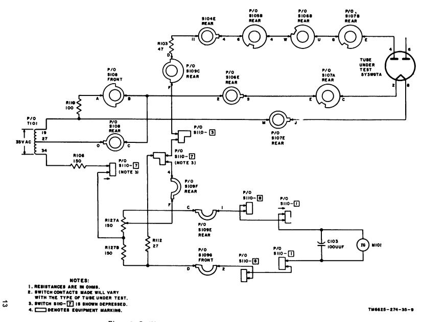
Figure 8. Rectifier test circuit, TV-7D/U, partial schematic diagram.
