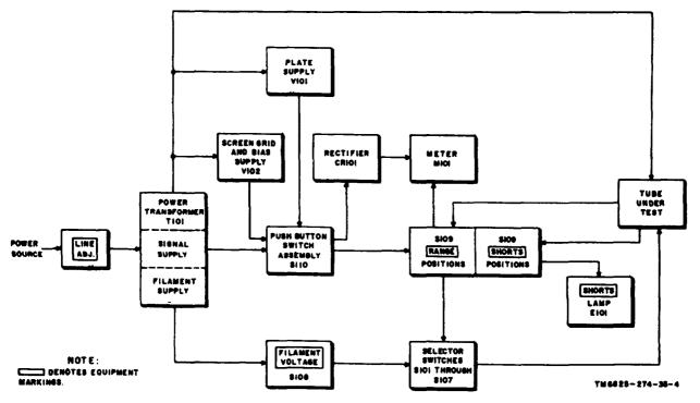
Figure 2. Test Set, Electron Tube TV-7(\*)/U, block diagram.
