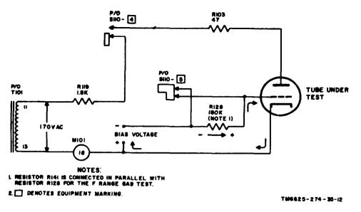
Figure 12. Simplified gas test circuit.
