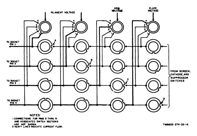
Figure 13. Simplified selector switch diagram.
