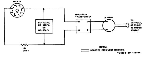
Figure 36. Connection for simulated tube test.
