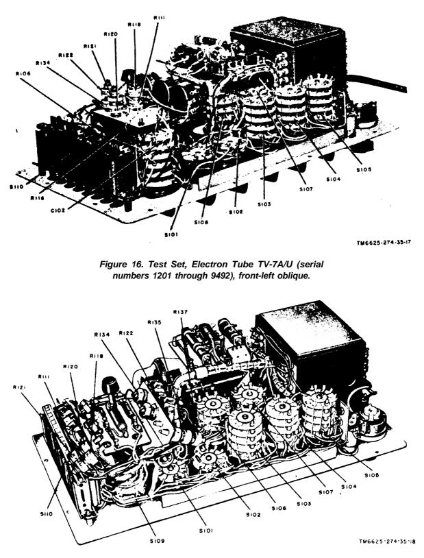
Figure 17. Test Set, Electron Tube TV–7BIU, front-left oblique.
