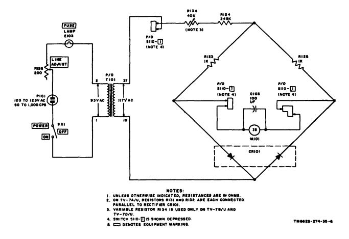
Figure 6. Simplified line voltage test circuit.
