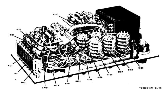
Figure 18. Test Set, Electron Tube TV-7D/U, front-left oblique.
