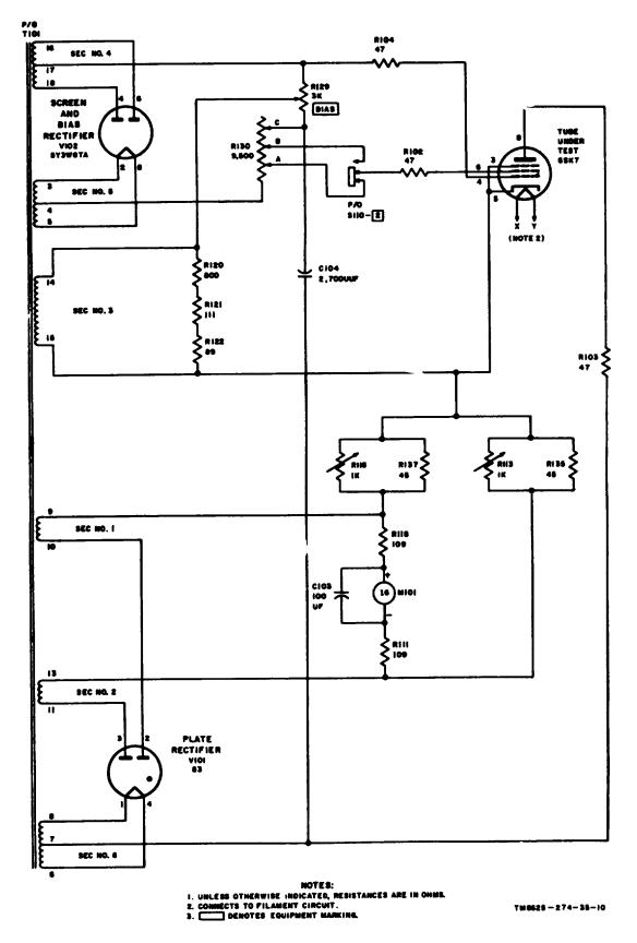
Figure 11. Simplified mutual conductance test circuit, TV–7D/U.
