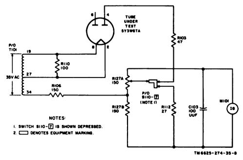
Figure 9. Simplified rectifier test circuit, TV-7D/U.
