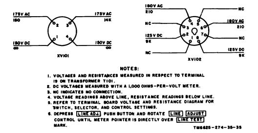
Figure 34. Tube socket voltage and resistance diagram.
