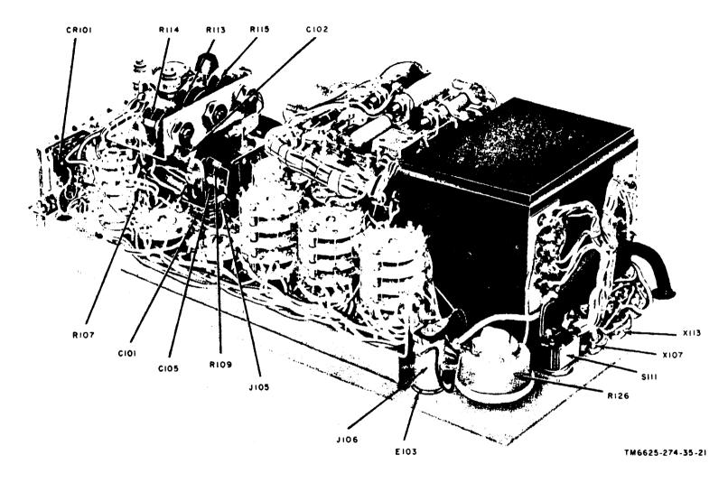
Figure 20. Test Set, Electron Tube TV-7A/U (serial numbers 1 through 1200), front-right oblique.
