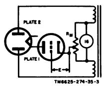
Figure 5. Basic mutual conductance circuit.
