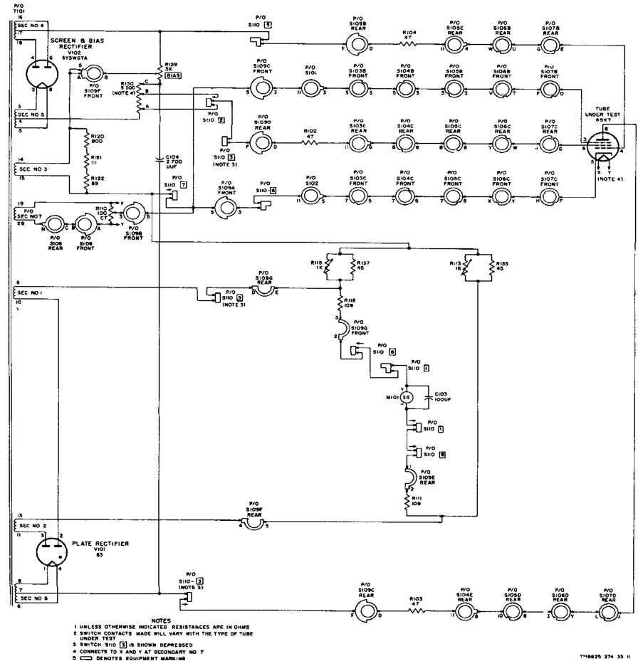
d. The partial schematic diagram (fig. 10) shows the various switch sections used and the Contacts made to test a type 6SK7 electron tube. Refer to the simplified circuit (fig. 11) for the operation of the circuit (e below).
