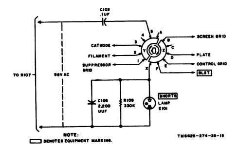
Figure 14. Simplified shorts test switch diagram.
