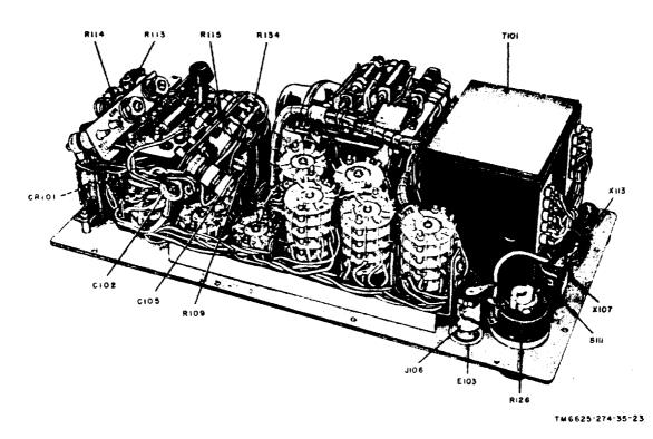
Figure 22. Test Set, Electron Tube TV-7B/U, front-right oblique.
