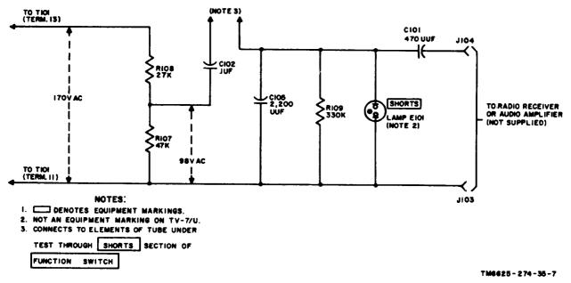
Figure 7. Simplified shorts and noise test circuit.
